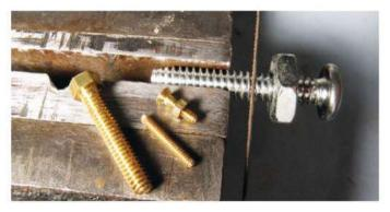
Unscrewing the nut over the freshly cut end of the bolt will straighten out any damage that sawing and filing did to the threads. Gripping the bolt by the piece to be sawed off localizes any crushing damage to the piece that will be thrown away.
