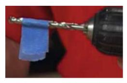
Note that a little extra tape left free on the end will blow away debris from the drilling
