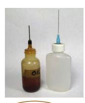
length of metal tubing on it. Plastics people use them for dispensing fast drying glues to join pieces of acrylic. The long metal tube let's you reach into tight places. Either of these is handy for flux at the soldering station.
