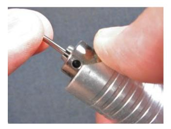
I have two ways to speed up that task. For opening up the jaws, I just remember "four", the number of turns I have to make to open the chuck just enough from the 3/32" bur shaft size to the larger 1/8" bur shaft size.
